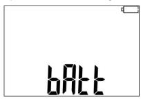
The battery pack is fully discharged,
